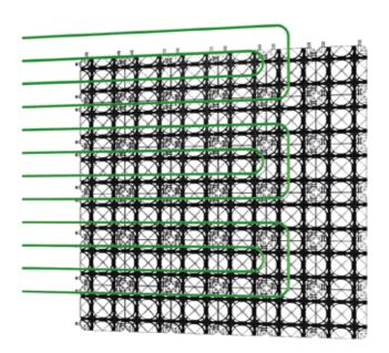
SpeeTile 10 is very suitable for wall heating (and cooling, in combination with a heat pump). The system's modular mats minimise installation height, which saves space. Due to its open structure, SpeeTile 10, in combination with a stucco layer, is very suitable for incorporation in walls.
